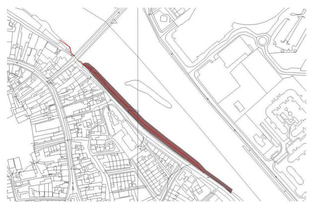
Figure 12 Construction Infill Area that includes for the Temporary haul road
