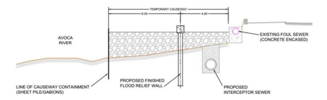
Figure 13 Cross Section through proposed temporary causeway
