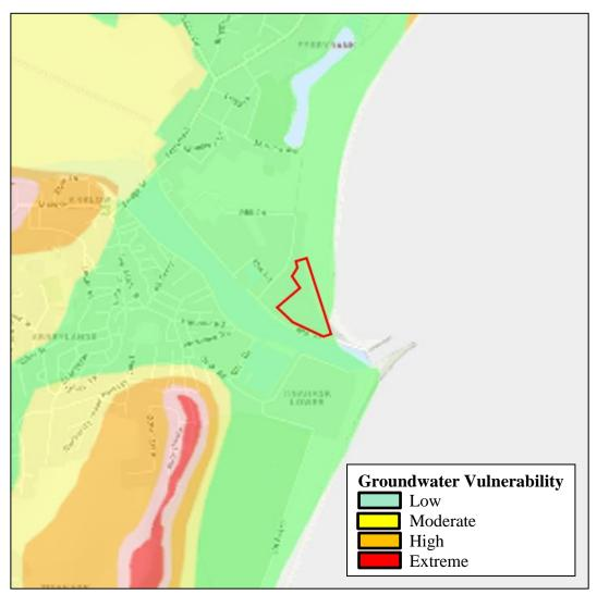
The Groundwater vulnerability maps indicate that the groundwater table may be high and/or the overburden may be reasonably permeable. This dataset however is only indicative and does not reflect the risk of groundwater flooding of the site.
