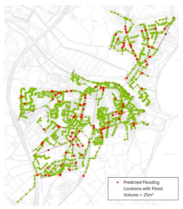
Figure 2: Existing System - Predicted flooding location > 25m3 for M30\_60 & MHWS with CC
