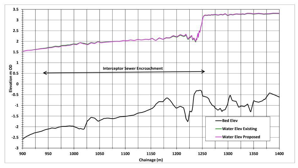
Figure 5: Computed Design Flood Profiles for the existing Case and proposed Sewer Encroachment Case
