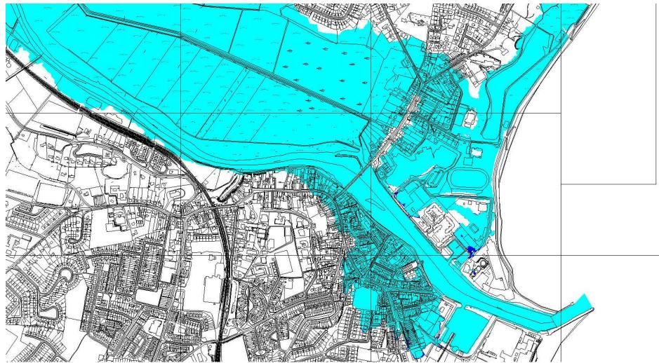
Figure 16: Predicted Flood Extents for existing and proposed temporary haul road downstream and Bridge arch underpinned and in-channel works completed at the bridge including upstream manhole encroachment. (Blue existing baseline and Cyan proposed construction) (overall minor reduction in the flood extents- very slight beneficial impact)
