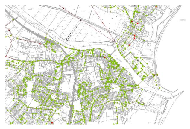
**Figure 7** Predicted flooding locations with flood volume >  $25 \text{ m}^3$  with all pumps down for M30\_60 & No tide
